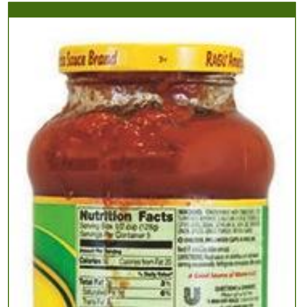
Signs of leakage
